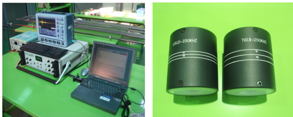
Fig. 3 Experimental setup of heat exchanger tube inspection system with MsS.
