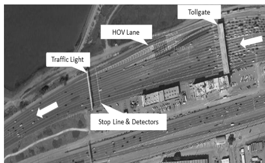
Figure 2. Mainline metering at toll plaza (Oakland Bay Bridge, San Francisco, U.S.)
