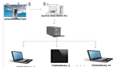
Figure 4: Concept of ultrasonic wind anemometer data-logger based Web
