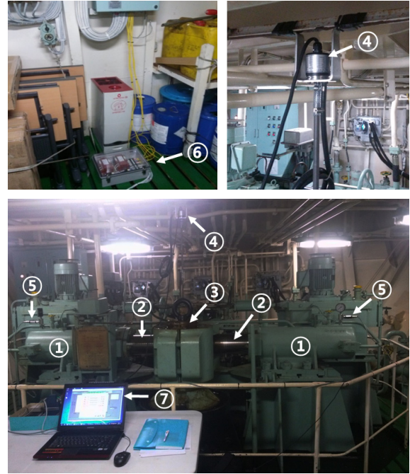
① cylinder, ② ram, ③ rudder tiller, ④ rudder angle sensor, ⑤ pressure sensor ⑥ electric power meter, ⑦ PC for data gathering
