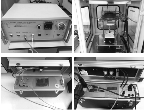
Fig. 1. Equipments used in this study(Thermal characteristic analyzer cone heater (ISO 5660-1/KS F ISO 5660-1) and NDIR analyzer).
