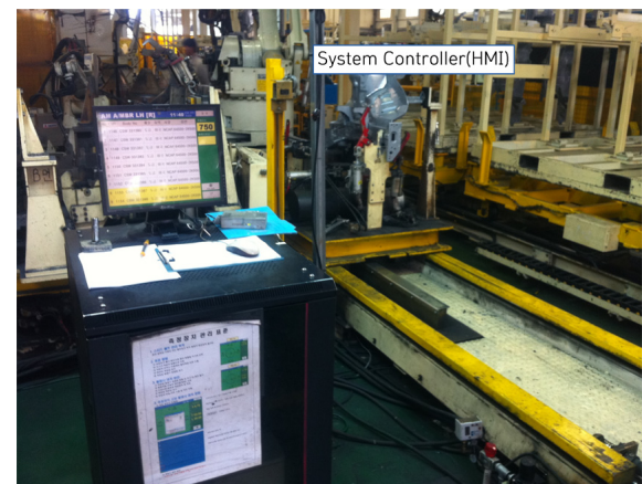
Fig. 3 Human machine interface for positioning and correcting system of stud bolt
