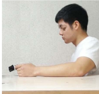
Fig. 1. The measuring position of HRV using pulse oximeter
