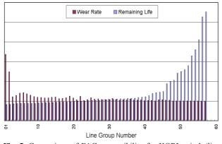
Fig. 5. Comparison of FAC susceptibility for KORI unit 1 (line group basis).
