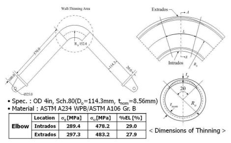
Fig. 9. Dimension of specimen for real scale failure tests.
