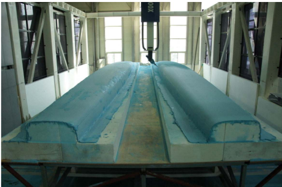
(a) Hull/Deck Plug Mold Using 5-Axis Machine
