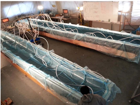
(b) Vacuum Infusion Method of Construction
