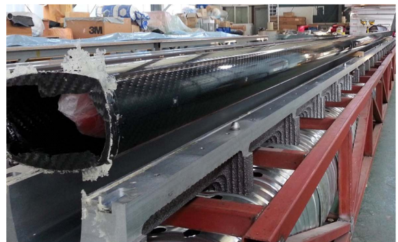
(a) Mast/Boom Metallic Mold
