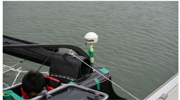
(a) Sea Trial Test Setting of DGPS
