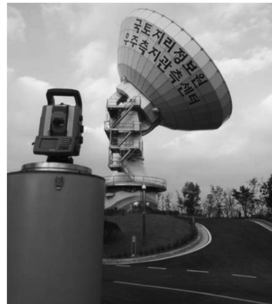
Fig. 4. The ground coordinate measurement method for feature points of VLBI antenna
