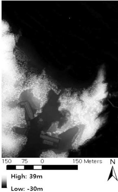
Fig. 5. One section of DSM generated using LiDAR point cloud
