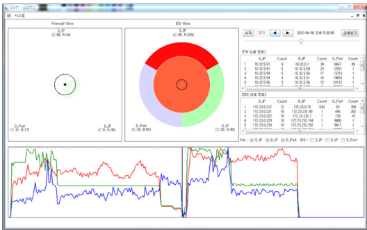
Fig. 14. Firewall or network switch failure 1
