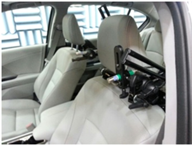
Photo. 1 Microphone setup for measurement
