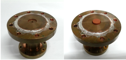
Fig. 4 Photograph of catalyst reactor without and with pellet-form catalyst
