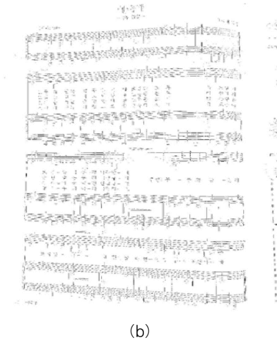
Figure 4. (a) Captured image, (b) Extracted edge image by using Sobel operator on blocks
