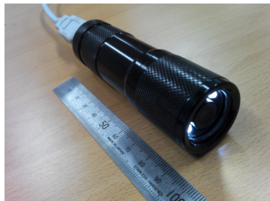
(Figure 6) Packaged camera module inside a cylindrical Aluminum case.
