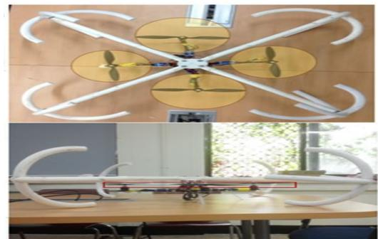
Fig. 3 Fabricated protective device shape and interference check with quadcopter
