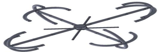
Fig. 2 3d model of quadcopter with protective device
