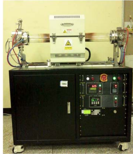
Fig. 1. Equipment thermal CVD used for graphene synthesis.
