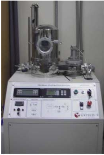
Fig. 3. Thermal evaporator for Metal thin film evaporation.
