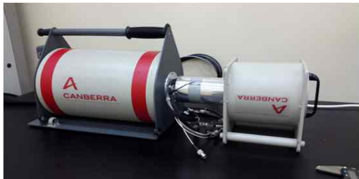
Fig 2. HPGe detector for measurement of delayed gamma ray from the Al sample.
