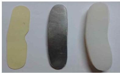
a. Bismuth b. Aluminum c. Silicone Fig. 1. Shielding materials.
