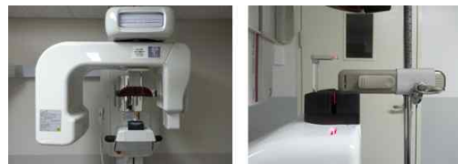
Fig. 1. Dental Panoramic X-ray System. (Left: Pax-400C system (Vatec Co., Korea, Right: Location of the Dosimeter in dental panoramic X-ray system)
