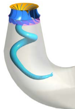
Fig.3 Vortex rope in draft tube
