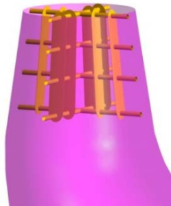
Fig.9 View of flow deflector
