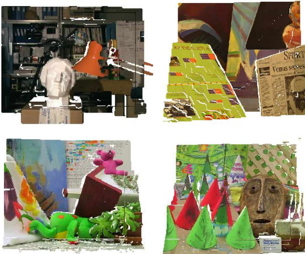
Fig. 9. 3D scene reconstruction results by using the produced disparity images.
