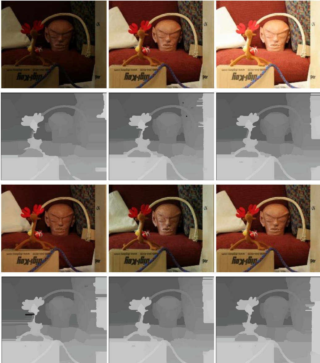
Fig. 7. Experimental results of the Reindeer pairs by the proposed method with radiometric difference. The first row are the left images under three different exposures and the second row are the corresponding disparity maps. The third row are the left images under three different light conditions with the corresponding disparity maps shown in the last row.
