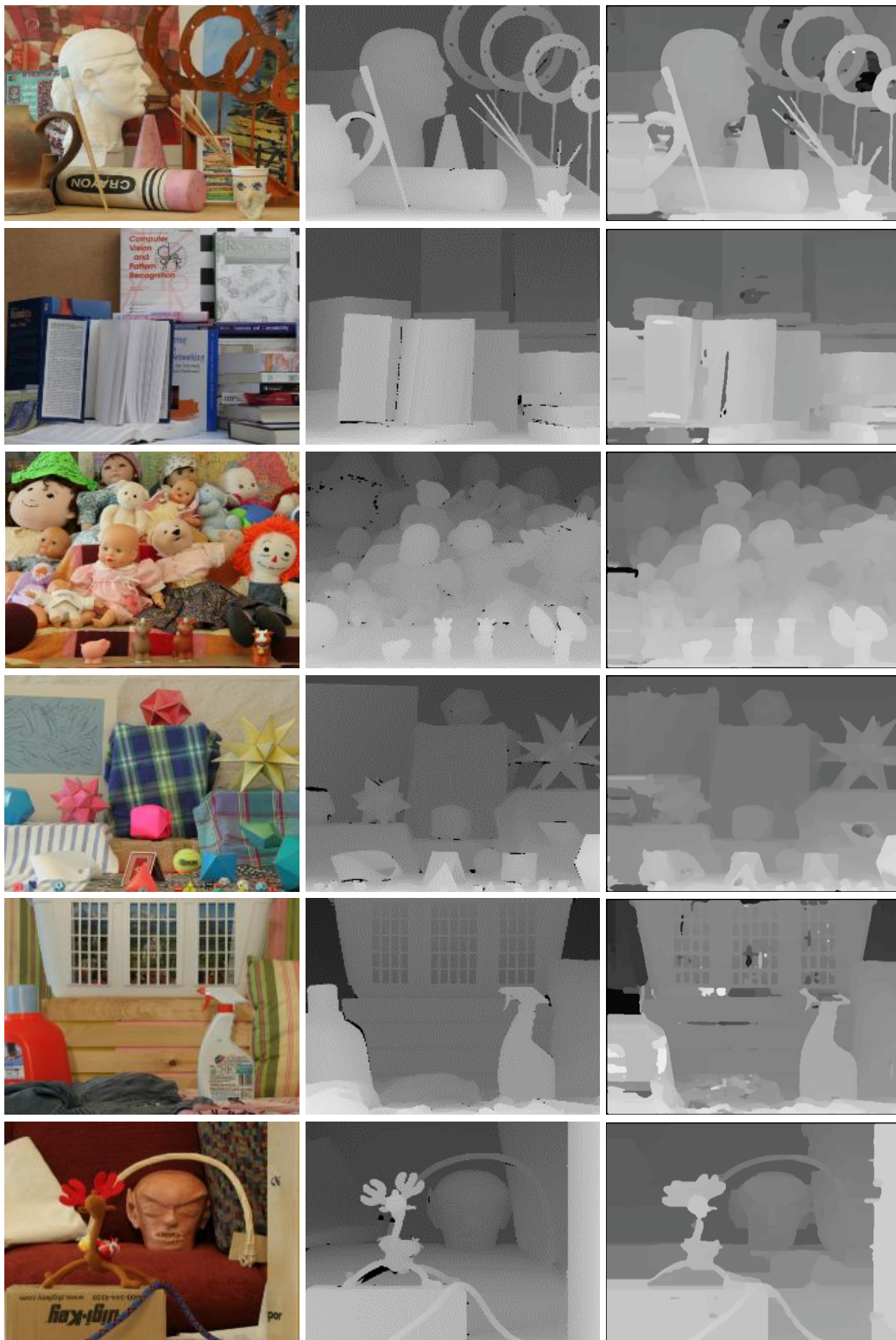
Fig. 6. More experimental results without radiometric difference. From top to down are accordingly the Art, Books, Dolls, Moebius, Laundry, and Reindeer stereo datasets. From left to right are the original color images, ground truth and disparity maps produced by the proposed method.
