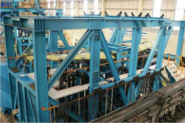
Fig. 5 Main Wing Durability Test Set-Up
