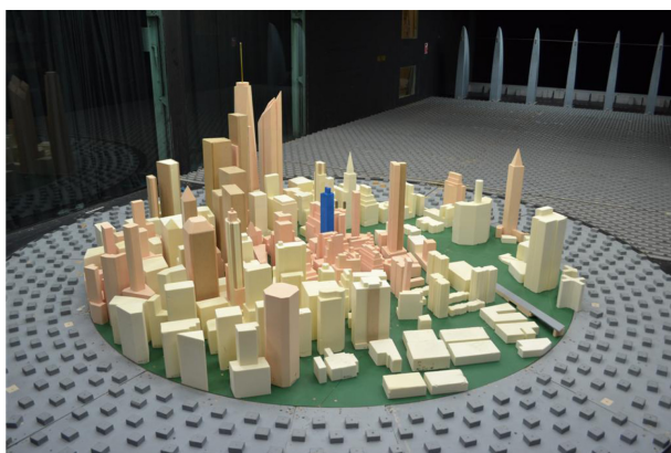
Figure 1. Test section of a wind tunnel [BMT Fluid Mechanics].
