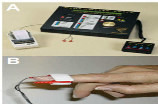
[Fig. 1] (A) Method of current perception threshold test. (B) A Neurometer ® CPT/C was used to measure current perception threshold (CPT) values at frequencies of 2000, 250, and 5 Hz in the right finger to assess the tactile sense, fast pain, and slow pain, respectively.
