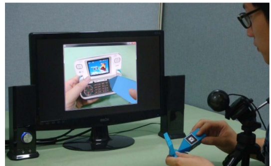
Fig. 10 Environment for AR-based virtual prototyping
