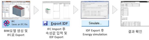
Fig. 5 BIM-based energy simulation process
