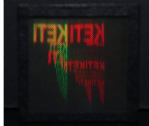
FIG. 13. A photograph of the reconstruction from a volume hologram printed with conventional mosaic recording.
