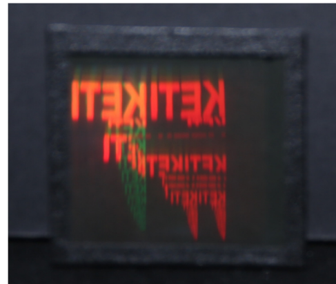
FIG. 14. A photograph of the reconstruction from a volume hologram printed with adaptive spatial partitioning of the SLM.
