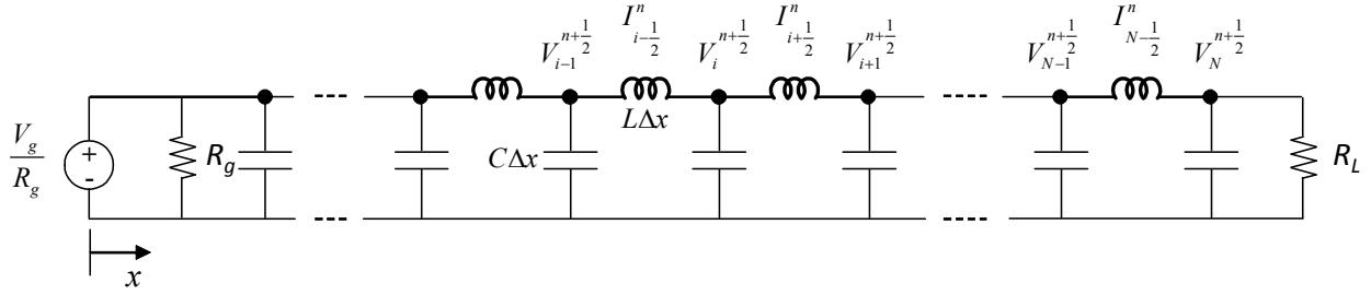
Fig. 3 LC distribution model for transmission line
