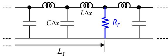
Fig. 4 Distribution model at leakage location,  $L_f$
