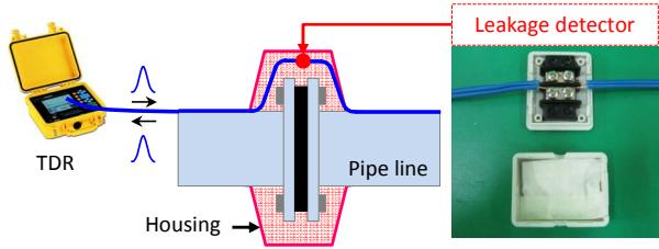
Fig. 2 TDR based pipe leakage detection system
