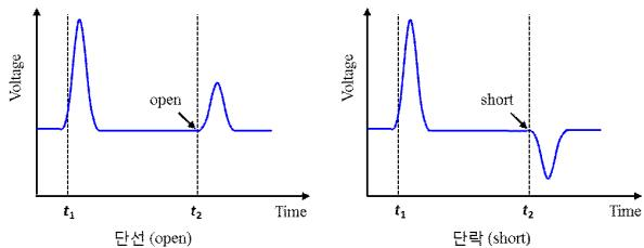
Fig. 1 Pulse response to the open and short of the cable
