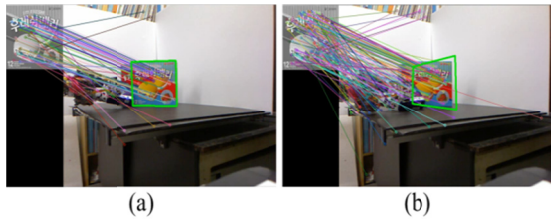
Fig. 2. (a): normal recognition of homography (b): abnormal recognition of homography
