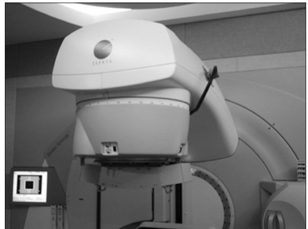
Fig. 1. Dynamic micro-multileaf collimator (DMLC) attached to the Elekta Synergy linear accelerator. The electrical connection between the DMLC and the gantry is established by only on cable.
