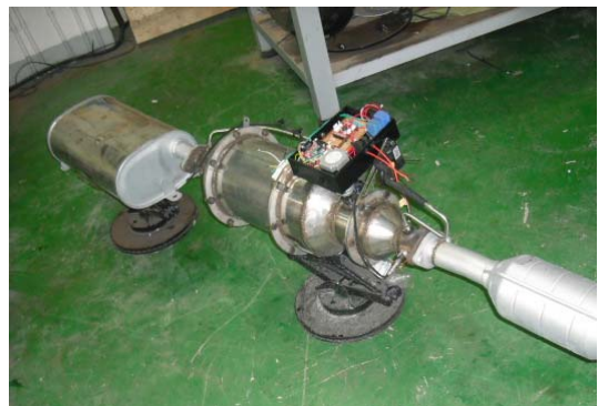
Fig. 3.3 2-Way installation of the exhaust system.
