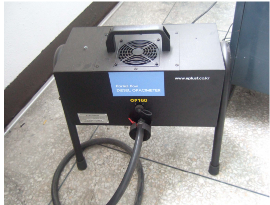
Fig. 3.2 Soot measurement instrumentation OP-160.
