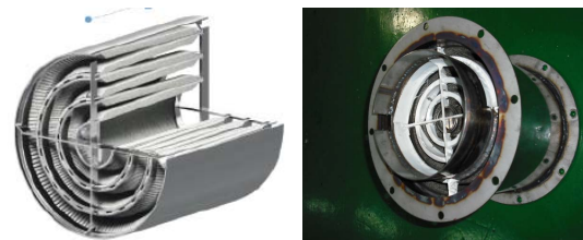
Fig. 2.7 Production of Ammonite Trap Filter.
