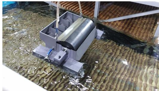
**Fig. 3.2** Oil skimmer tests on wave height
