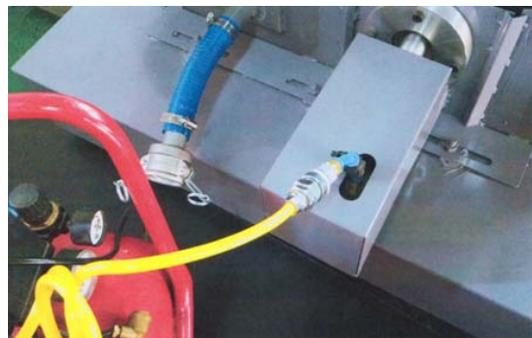
**Fig. 3.3** Air motors and skimmer continuous operation test
