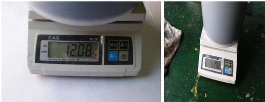
**Fig. 3.1** Weight of the bunker oil before the test skimming (14.21L), after the test (13.85L)
