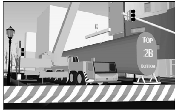
Figure 13 Planned site logistics for the final pick of the connector bridge as developed using BIM
