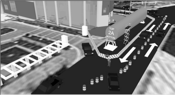
Figure 8 3D view of logistics plan during the 10 days of preparatory work between offload and installation
