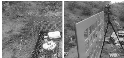
(a) Setting the Thermocouple (b) Setting the thermo-graphic camera
