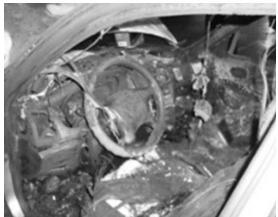
Fig. 2. Fire example producing by overheat of clutch.
