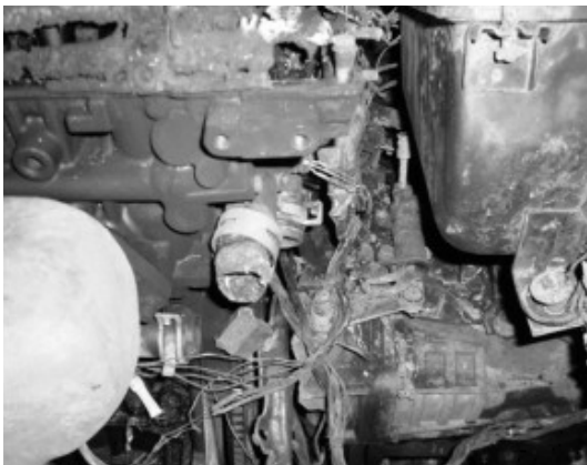
Fig. 3. Fire example by leaking of manual transmission fluid.
