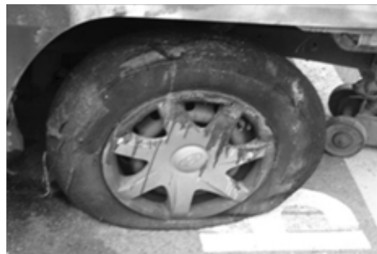
Fig. 4. Fire example by friction heat between tire and road.
