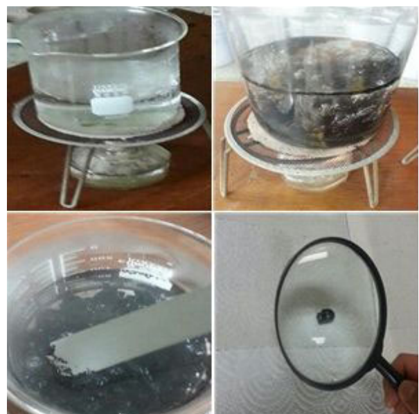
Fig. 2 Procedures for Boiling Water Test
