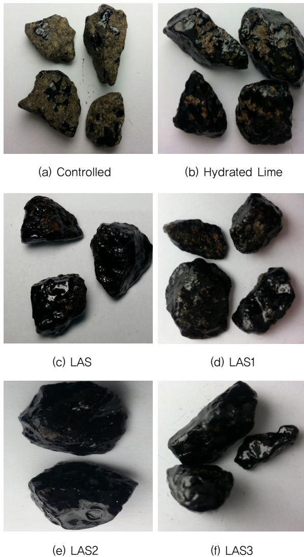
Fig. 5 The Results of Stripping of Coated Aggregates after Boiling Water Test
