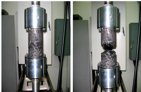
Fig. 4 (a) Bond Strength Test Set-Up and (b) Specimen After Testing
