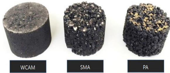
Fig. 3 Prepares Asphalt Mixtures (with EAF steel slag)
