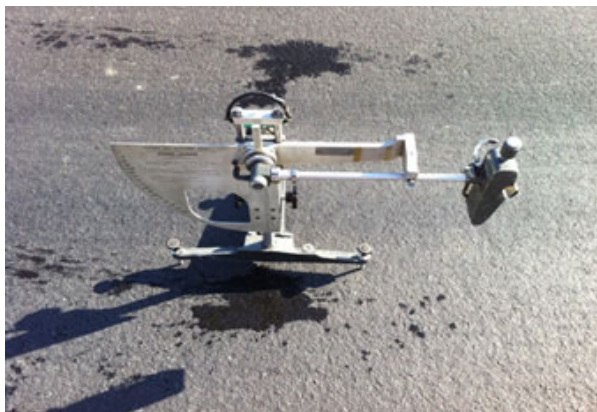
Fig. 5 Skid Resistance Tester (British Pendulum Test)
