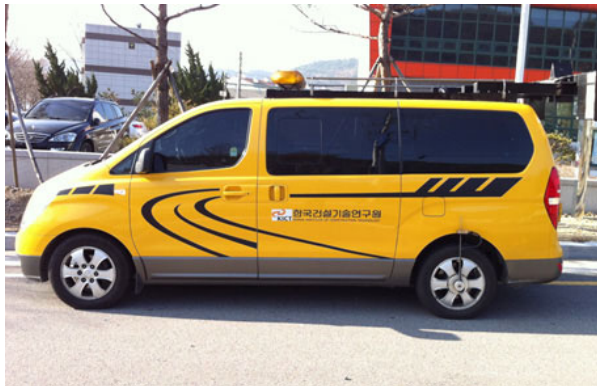
Fig. 4 Automatic Surface Condition Surveyor (PES, Pavement Evaluation Surveyor)
