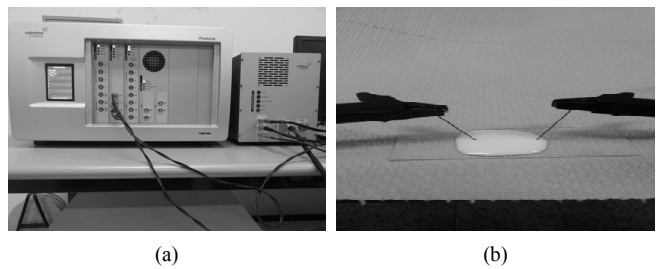
Figure 13. (a) Experimental setup for conductivity measurements. (b) Photograph of probe-station setup showing crushed microcapsules on a glass substrate.
