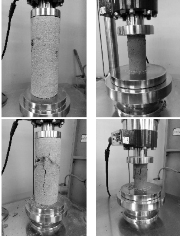
(a) Cemented with Portland ordinary cement (b) Cemented with microorganism
