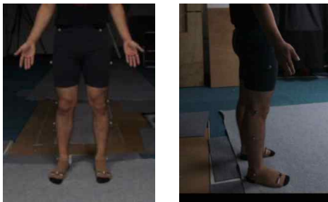
Figure 2. Attachment of the reflective markers
