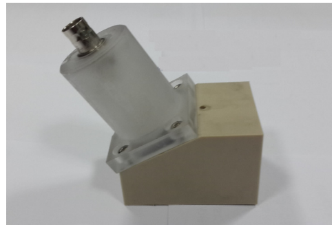
Fig. 6 Prototype of an ultrasonic transducer
