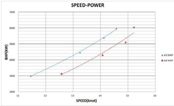
Figure 5: Speed-Power for A3 ship and A4 ship
