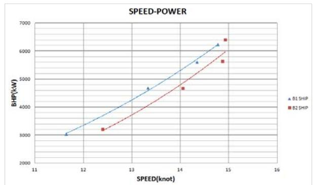
Figure 10: Speed-Power for B1 ship and B2 ship
