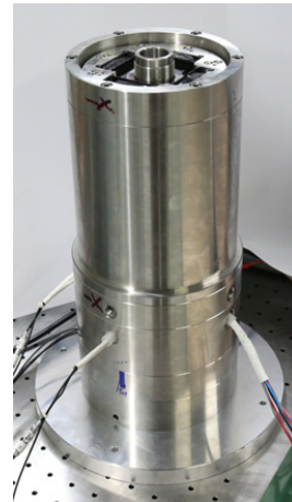
Fig. 12 Assembled high speed spindle with magnetic bearings
