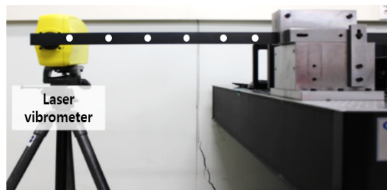
Fig. 4 Modal test for the cantilever beam
