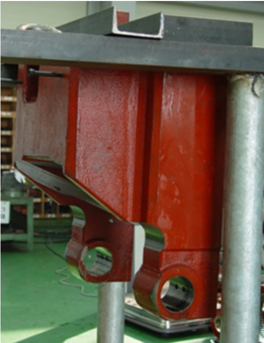
Fig. 5 Manufactured counterbalance weight after dynamic balancing. Mass is 344 kg
