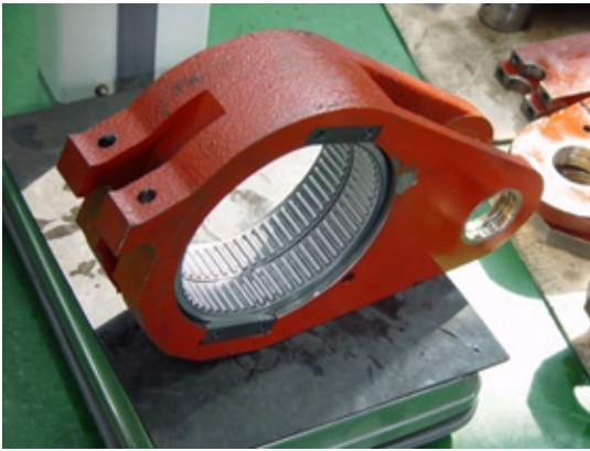
Fig. 4 Manufactured connecting rod after dynamic balancing. Mass is 50.5 kg. Two identical connecting rods are used. Refer to Fig. 2(a)
