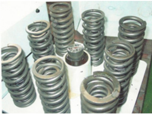
(a) One of 4 isolation systems installed underneath the 4 legs of the press. A viscous damper is located at the center and using silicone oil
