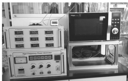
Fig. 1. Microwave radiation facility for thermal desorption treatment of bunker fuel oil C contaminated soil.
